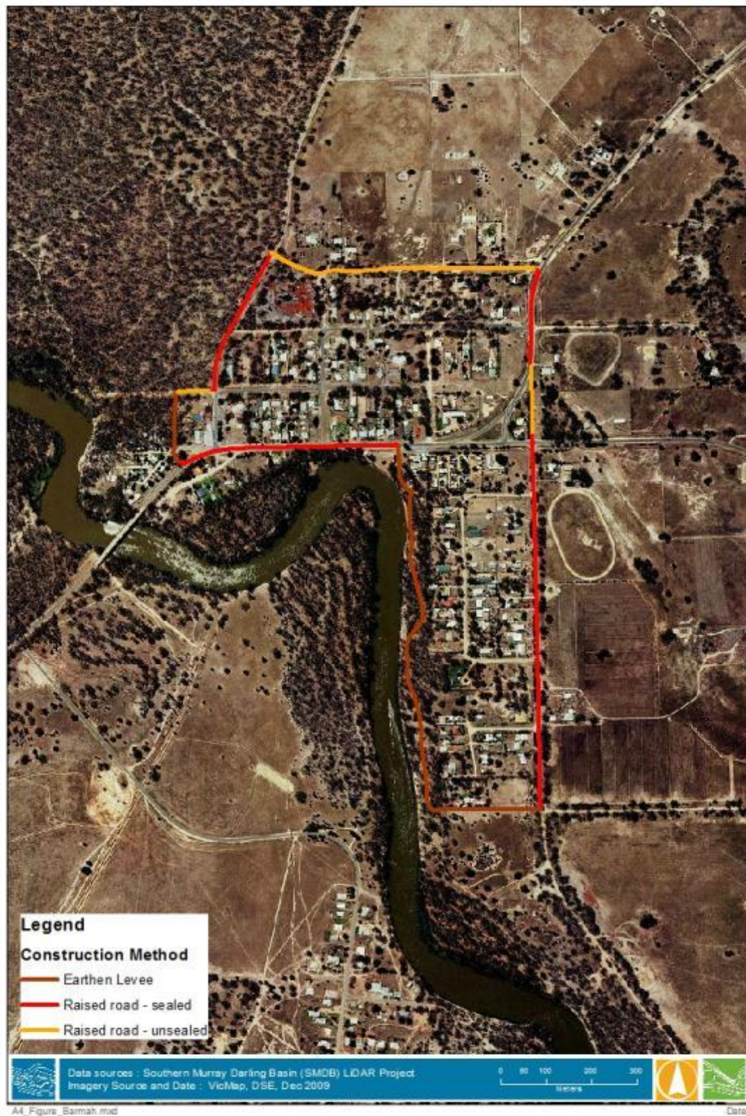
Figure 13 Preferred Levee Alignment and Construction Method
